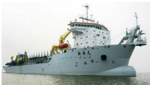
13500m 3 耙吸挖泥船 13500m 3 Trailing Suction Dredger
