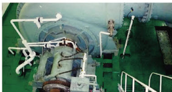
中交天津航道局滨海3000项目部3号船 800WN型舱内泵 800WN inboard Pump In 3rd Dredger Of Project Binhai 3000 Of CCCC Tianjin Dredging Company
