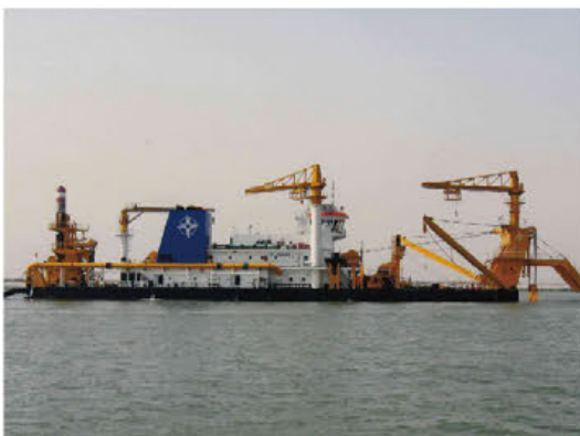
中交天津航道局天风号挖泥船作业现场 On Site Operation Of The Tianfeng Dredger From CCCC Tianjin Dredging Company
