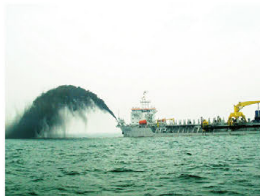
中交天津航道局11000m 3 耙吸挖泥船 11000m 3 Trailing Suction Dredger From CCCC Tianjin Dredging Company
