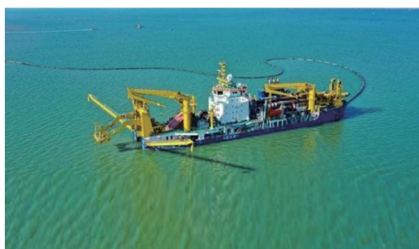
Asia's Largest Heavy Self-propelled cutter Suction Vessel "Tiankun"
